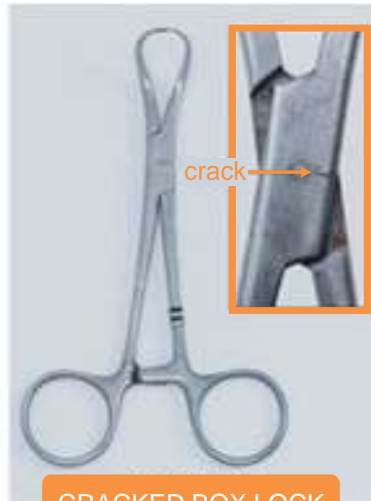
CRACKED BOX LOCK
