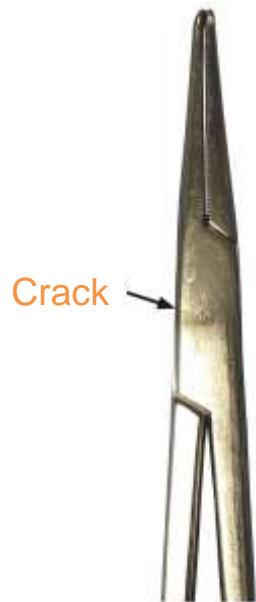
CRACKED BOX LOCK
