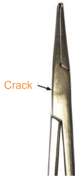
CRACKED BOX LOCK
